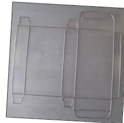
Top flexible die incl. creasing rules
